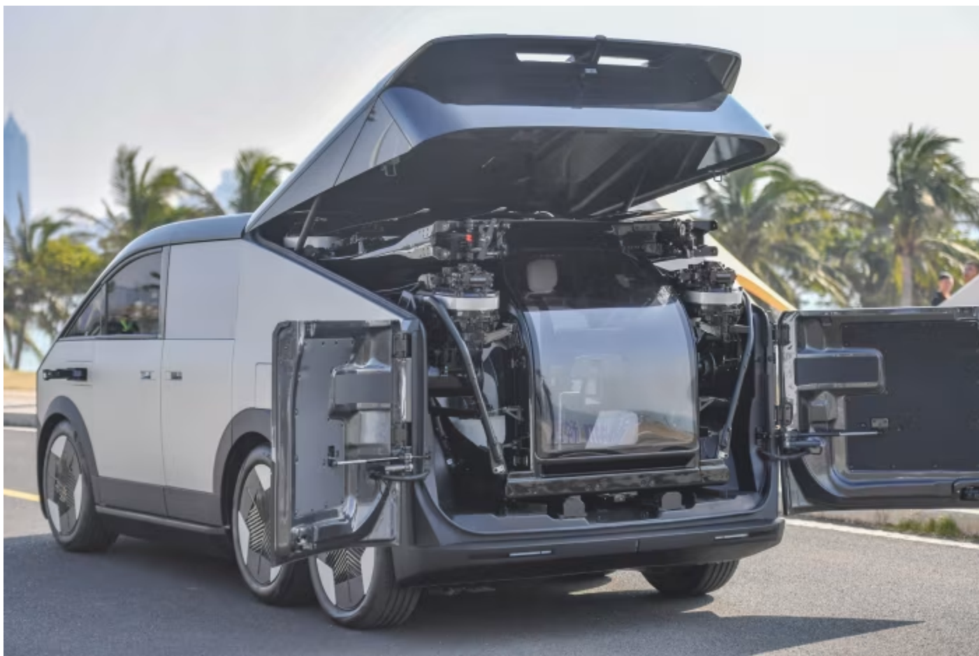
Xpeng's Land Aircraft Carrier, a van with a two-seat, battery-powered helicopter attached © Sun Shijie/VCG/Getty Images
